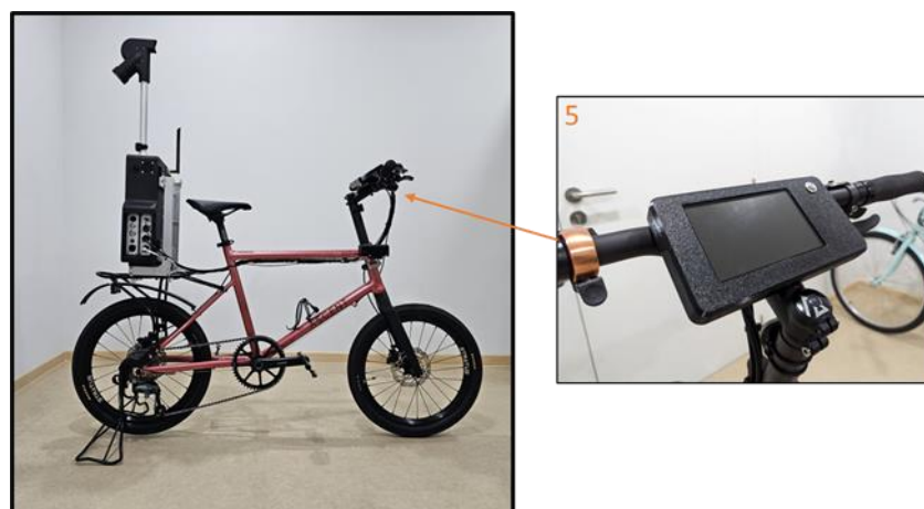
Figure 5 PathWatcher Front-end Unit in bike-mounted configuration, securely mounted onto a lightweight bicycle with custom designed mountings, equipped with (5) touchscreen panel.
