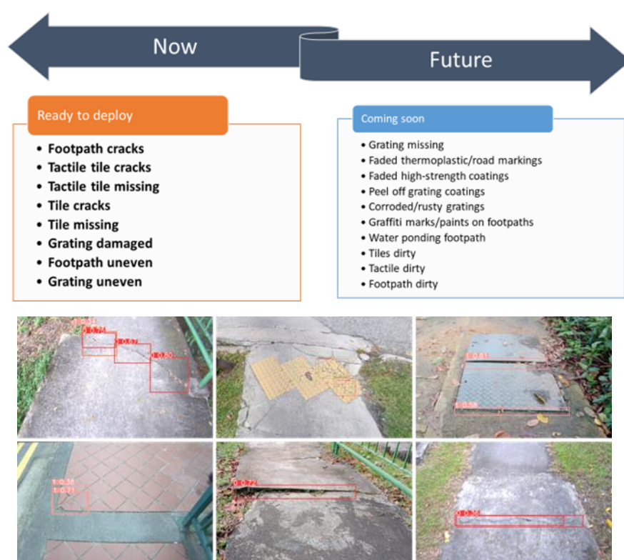
Figure 9 List of defect types currently detectable by the AI model and planned defect types in active development (top), images of pavement defects detected by AI model (bottom).
