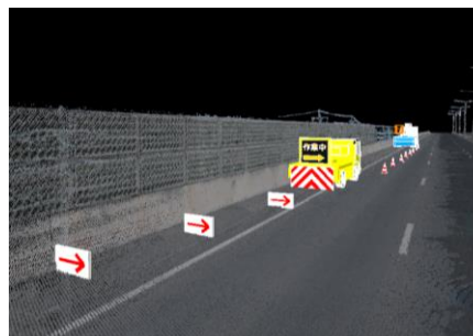
Figure 17 Simulation of work zone traffic control.
