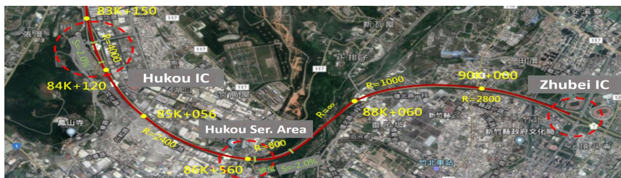
Figure 13 Hukou IC Nearby Mainline Southbound VD Data Analysis Schematic Diagram
